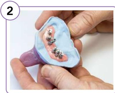
2 Apply soft tissue replacement approx. 1–2 mm on the analogue. This enables us to visually inspect the fit.
